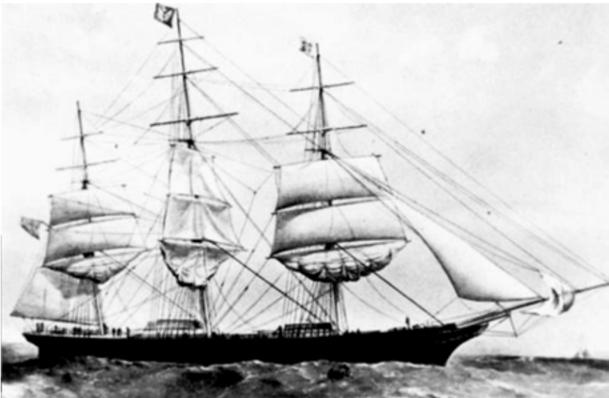
The Lammershagen had been built in Scotland in 1869. Constructed of iron and with three masts, its length was 182ft. It was owned by R.M. Sloman Jr. of Hamburg, and was lost in 1882.
